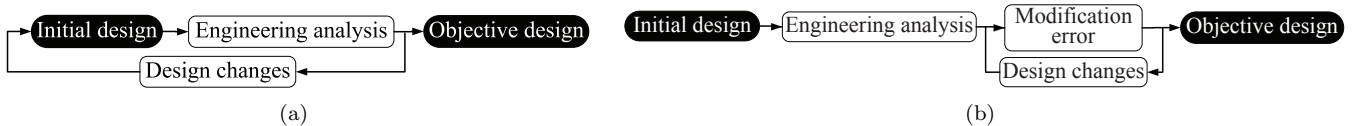
Fig. 1. Different strategies for simulation-based design. (a) repeated engineering analysis is required for each design change; (b) using modification sensitivity estimation, only one step of engineering analysis is required for all model modifications.
