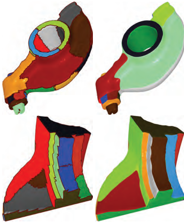
Fig. 8. Segmentation of engineering objects: rocker arm and fan disk. Left: initial segmentation with fine-scale seeding. Right: results after merging and smoothing.
