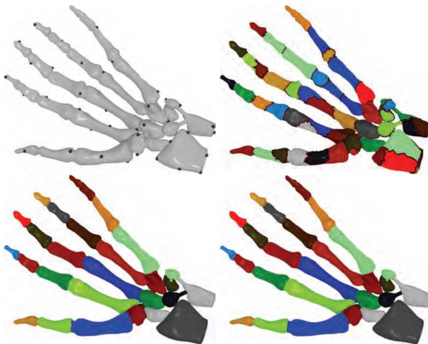
Fig. 5. Example of fine-scale seeding. From top left to bottom right: input model with automatic seed selection; initial (over-) segmented results; result after merging; final result after boundary smoothing and mapping.
