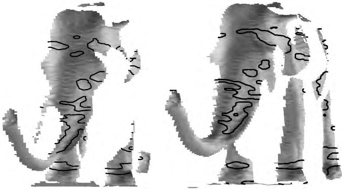
Figure 3: The range images obtained from two different view directions with extracted intrinsic curves.
