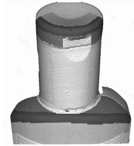
Figure 19: Segmentation of data into primary and blend surfaces
