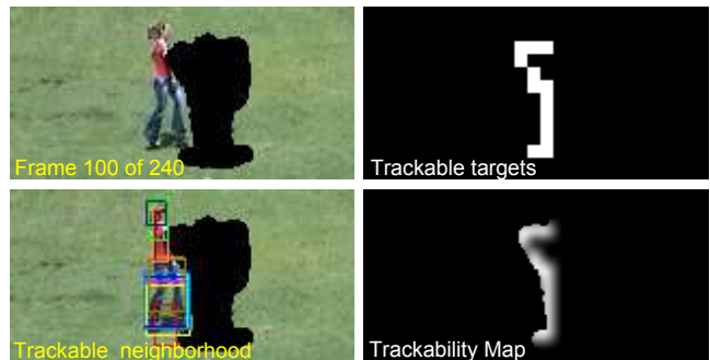
Fig. 4 From top left to bottom right: source frame, trackable target fragments, trackable neighborhoods of target fragments, trackability map of source frame.
